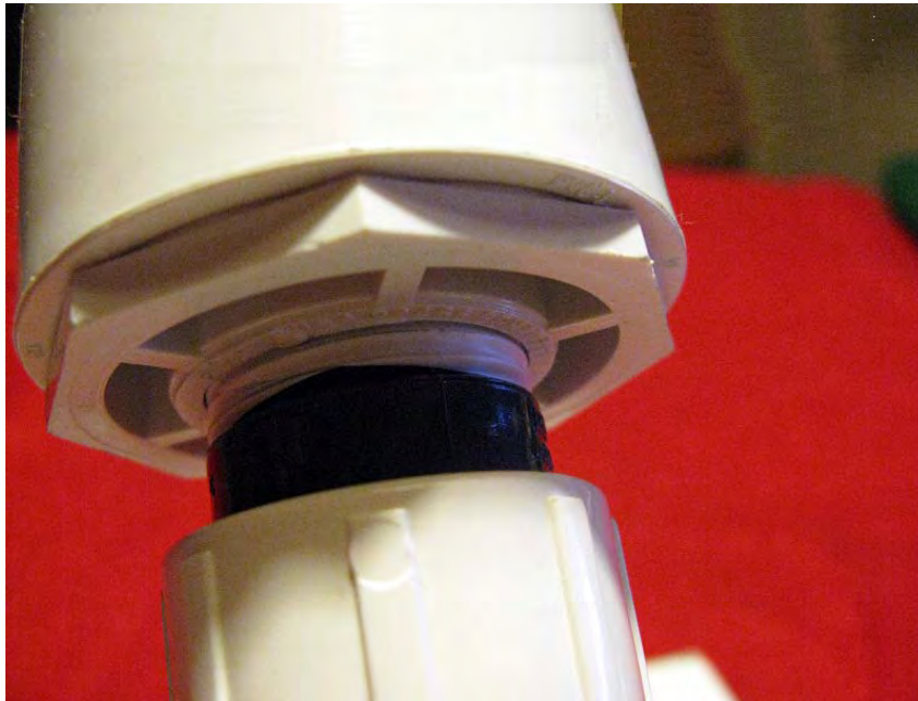
This is a bubbler constructed from "Whole Household Prefiltration" units supplied by Home Depot, which unfortunately, may cost more than US $100 each.
