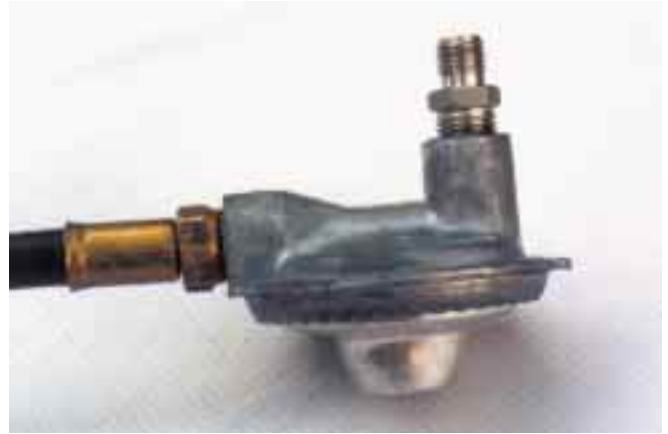
Above: The gas pressure regulator with Swage lock tubing INLET pipe fitting.
