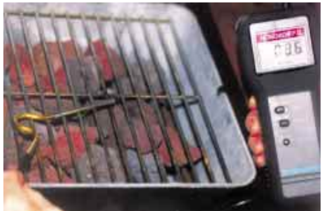
Above: Test setup showing barbecue, NOx meter at 50% hydrogen flow (86 ppm)
