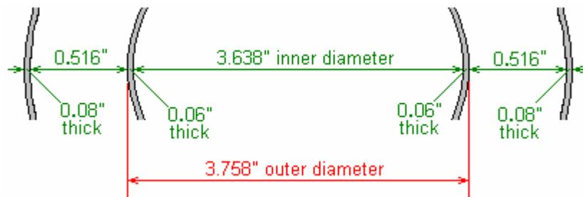
The length of stainless steel needed to form that cylinder will be the circumference of the outer diameter of 3.758" which will be 3.758" x 3.1415926535 = 11.806 inches.
