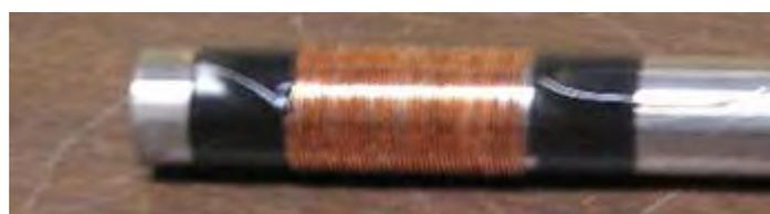
The wire for the second layer is cut to a length of 396 centimeters. This second coil layer will be longer than the first layer, so before winding it, it's necessary to build up the area at both ends of the first layer with tape:
