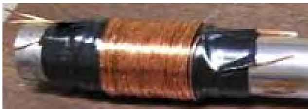
To be sure that the second and third layers are centred over the earlier layers, it is a good idea to locate the centre of the wire and start winding from the middle outwards in both directions:
